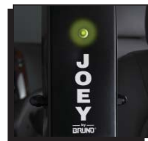
Visible docking indicator light (ready to charge)
