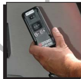
On/Off switch in the pendant NOW turns off the controller (main circuit board) to maintain battery charge. However, the "charging circuit" is still active. This feature eliminates all battery drain from the motor control circuitry, preventing battery discharge during long unused periods.
